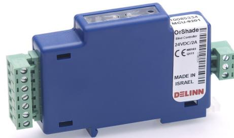
On the hardware side the 9201 and 9206 is designed with low-power technology and consumes as little as 0,5 Watt. The dry-contact inputs can be configured to act as master of groups of blinds on the databus.
